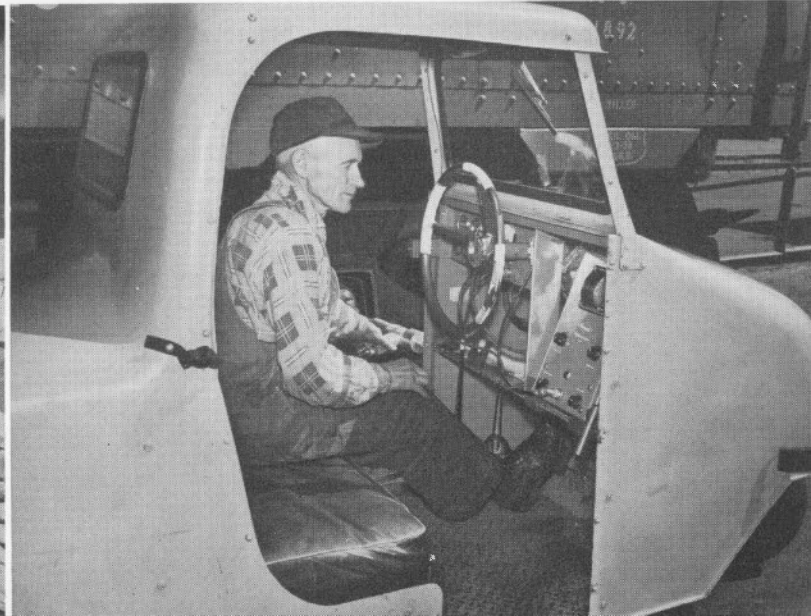
The Reflectoscope screen is situated in a nearby mobile unit, where the condition of axles can readily be interpreted from the projected images.
