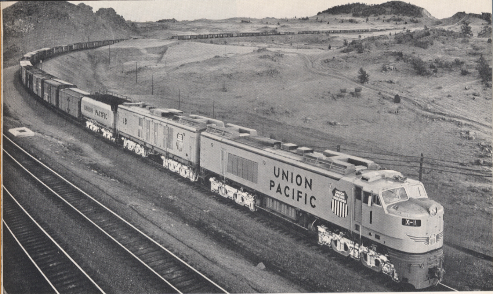
New 8,500 H.P. Gas Turbine Electric Freight Locomotive, Westbound to Laramie, Wyoming.
