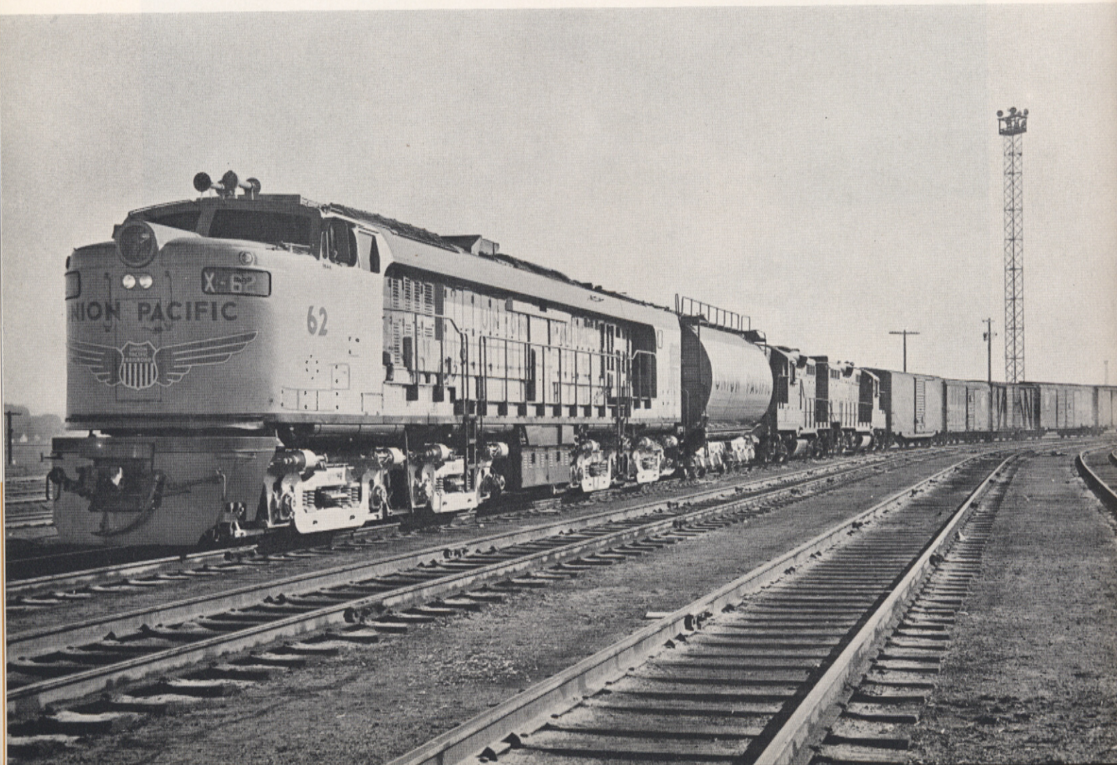
Combined Power — Gas Turbine Electric and Diesel Locomotives in Tandem.
