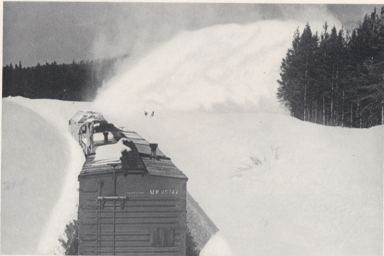
Union Pacific-Built Snow Plow in Use on the West Yellowstone Branch.
