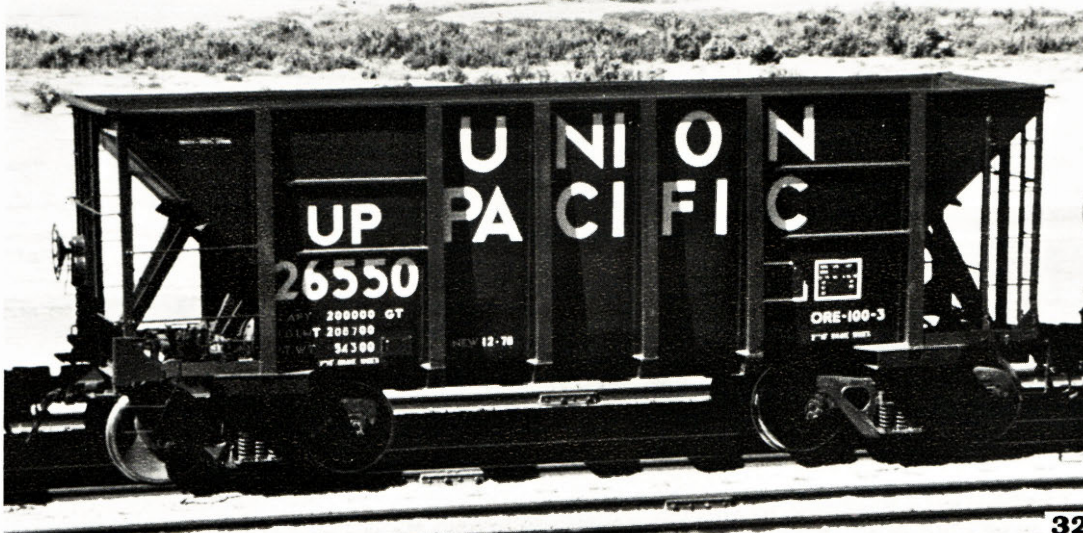
26550 , class ORE-100-3, is one of the 250 new ore cars built by U.P. in Portland, OR. As seen here at Winton Junction, WY, 9.17 miles north of Rock Springs, WY at the junction where U S Steel exchanges their loads for the empties U.P. delivers. This exchange happened on September 4, 1979. Photo by G. B. Davies
