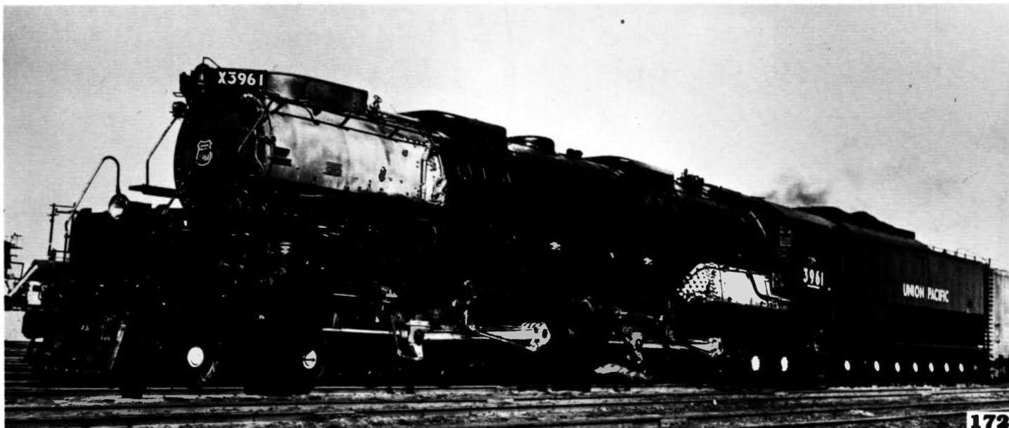
3961 is seen here ready to depart somewhere for someplace in a direction unknown. It is not brand new but evidently has been recently repainted. The locomotive is a CSA-3 class 4-6-6-4 Challenger. Photo courtesy Union Pacific Railroad
