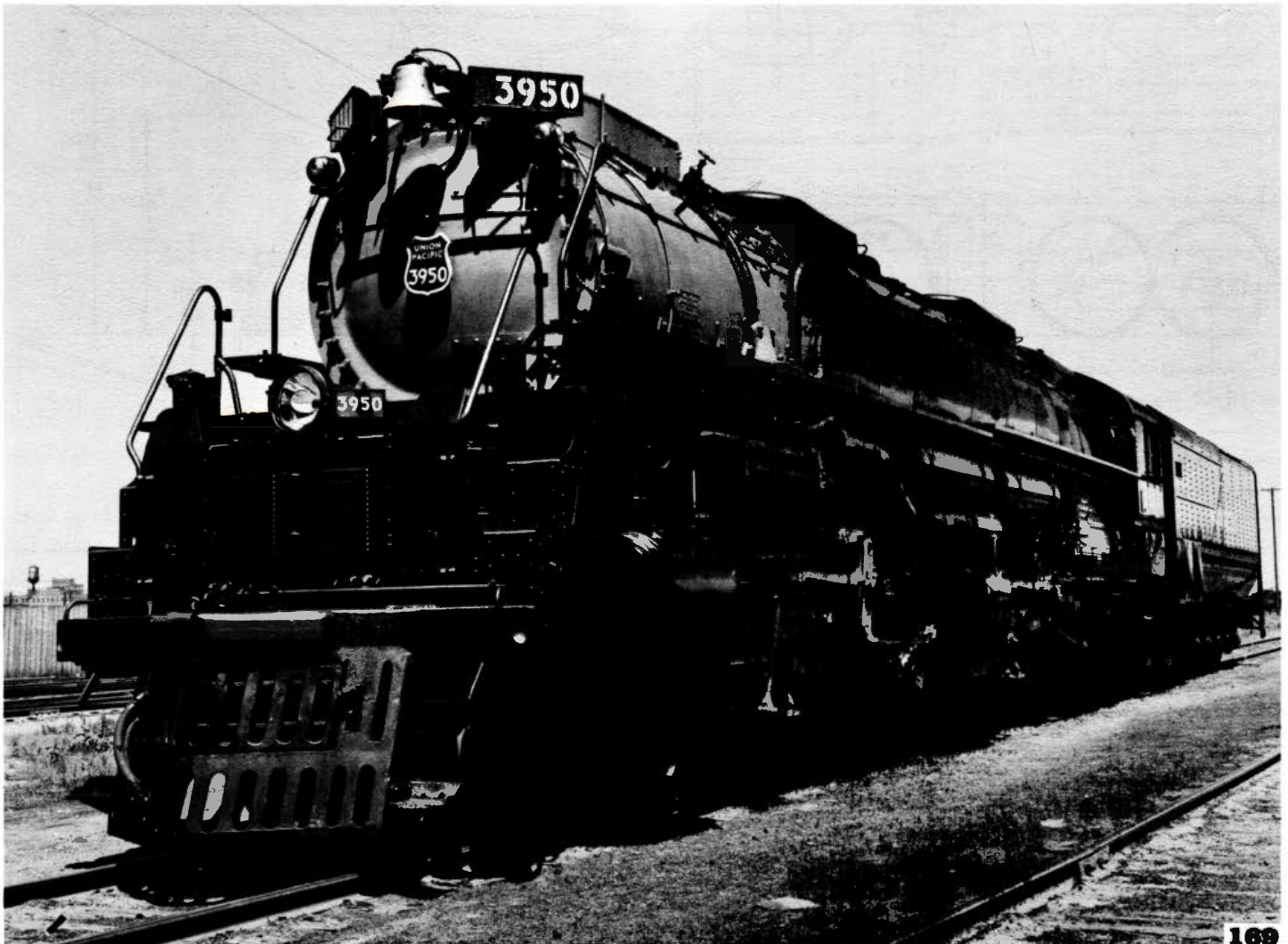
Another view of 3950 shows a little more just how big these steam locomotives really were. Consider the driver diameter was only 69 inches - or just under 6 feet high! Photo courtesy Union Pacific Railroad
