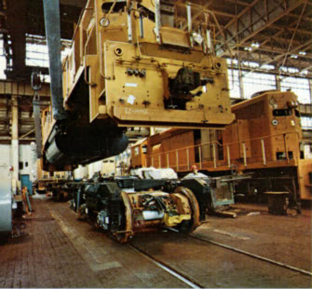
Left —A 3,000-HP road freight locomotive, part of Union Pacific's 1974 order, is shown under construction at the General Motors Electro-Motive Division plant in La Grange, Ill. General Electric is also a major supplier of locomotives for the Railroad.
