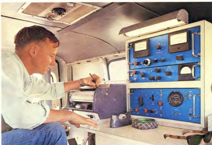
Field instruments recording seismic data for exploration.
