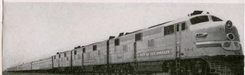
The Union Pacific's latest 18-car, 6000 horsepower Diesel electric streamliner, the "City of Los Angeles".
