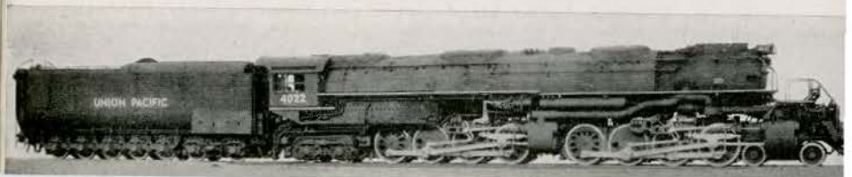
The "Big Boy", world's largest steam locomotive, which does the work of two locomotives. The Union Pacific has 25 of them.
