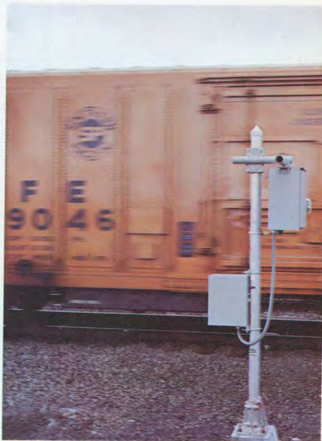
The scanners can read the identification plates three times as the train goes by at any speed up to 80 m.p.h.
