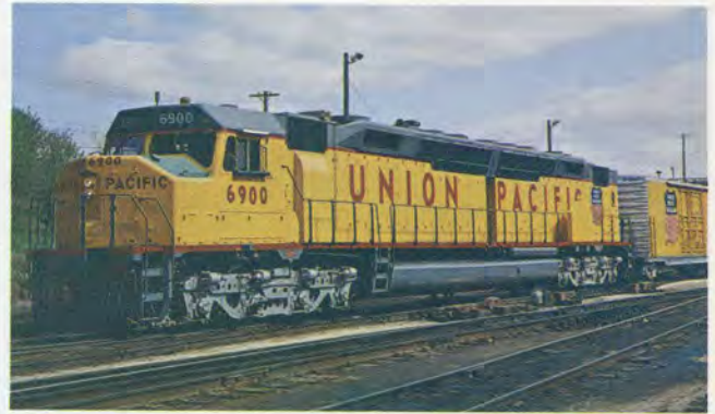
UP's 6,600 horsepower CENTENNIAL types are the giants of the diesel locomotive world.
