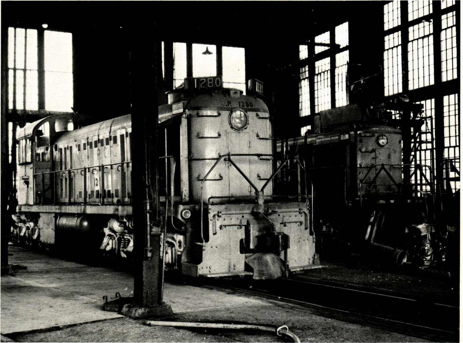
28 Two Alco switchers, 1280, an RSC-2 and 1120, an S-2, are receiving some minor repairs during their last days in service as switchers for the Cheyenne, WY yards. Photo by A. J. Wolff.
