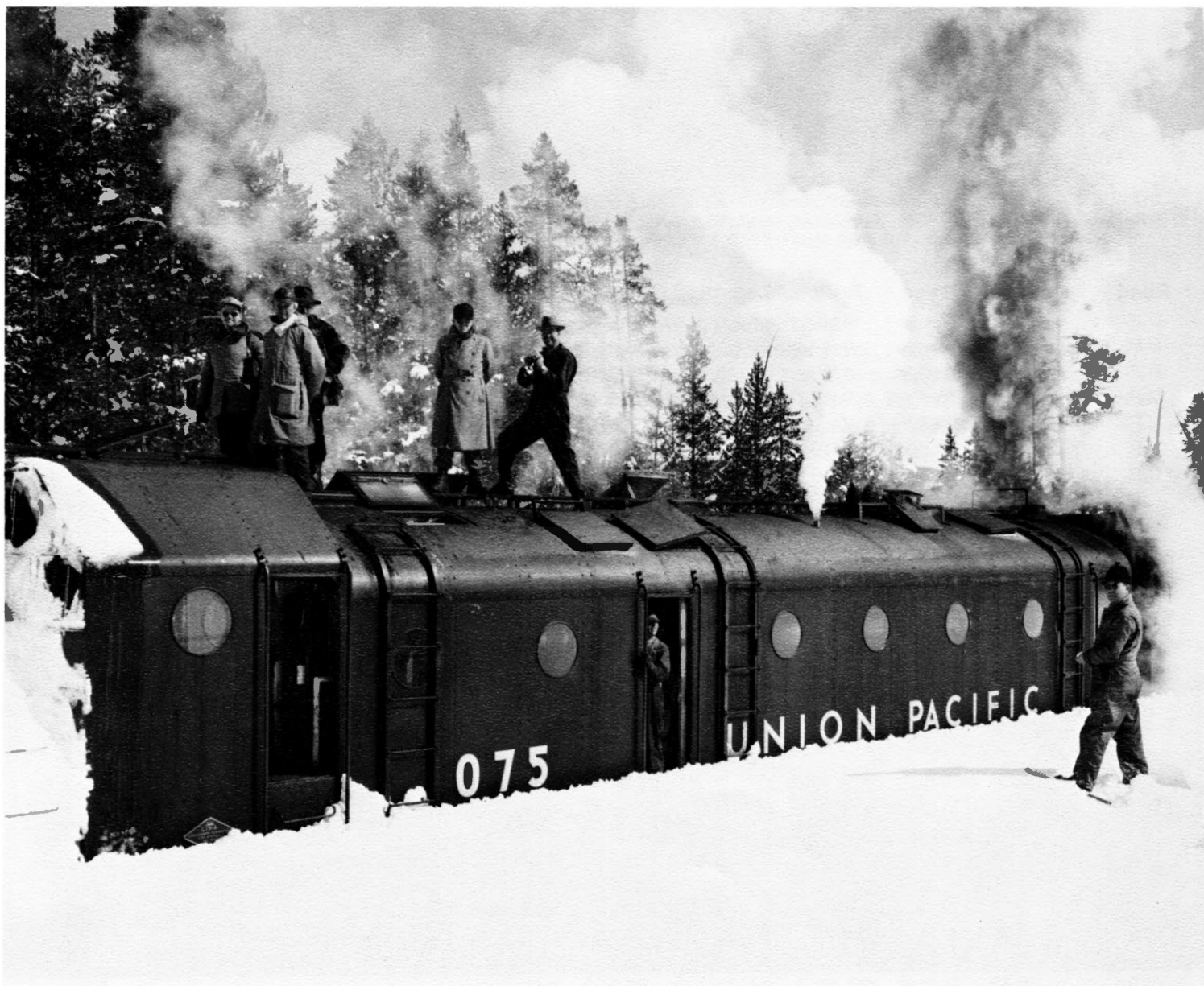
10 A close-up of Rotary Snow Plow 075 , built by Lima-Hamilton in January, 1950, shows some of the details of this Lima production. The event was the opening of the Yellowstone Branch in the spring of 1952. This is one of the tests given each new rotary and the reason so many people are present.
