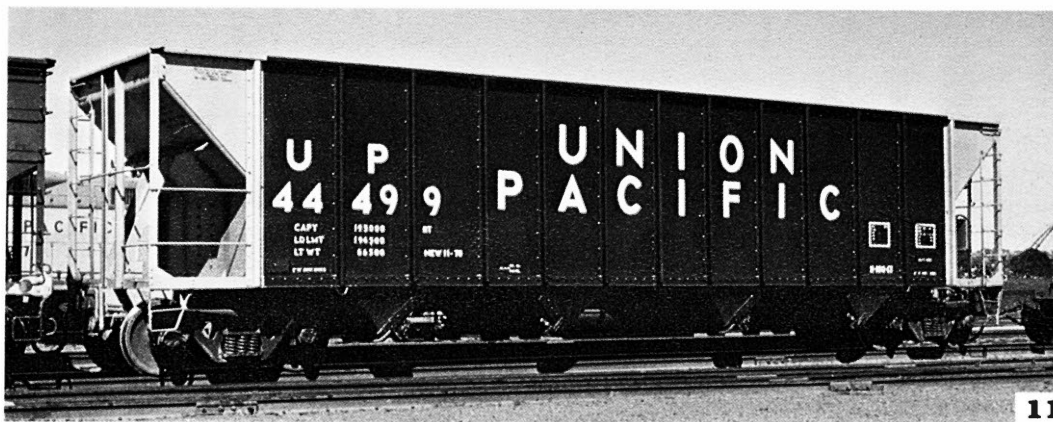
44499 class H-100-17 is the identical sister to 44498, both of which are the last two cars in the class of 500 cars built by the U.P.R.R. in 1978 and 1979 at their Albina, OR car shops. These two cars were the only two of that class to have double rotary ends.
