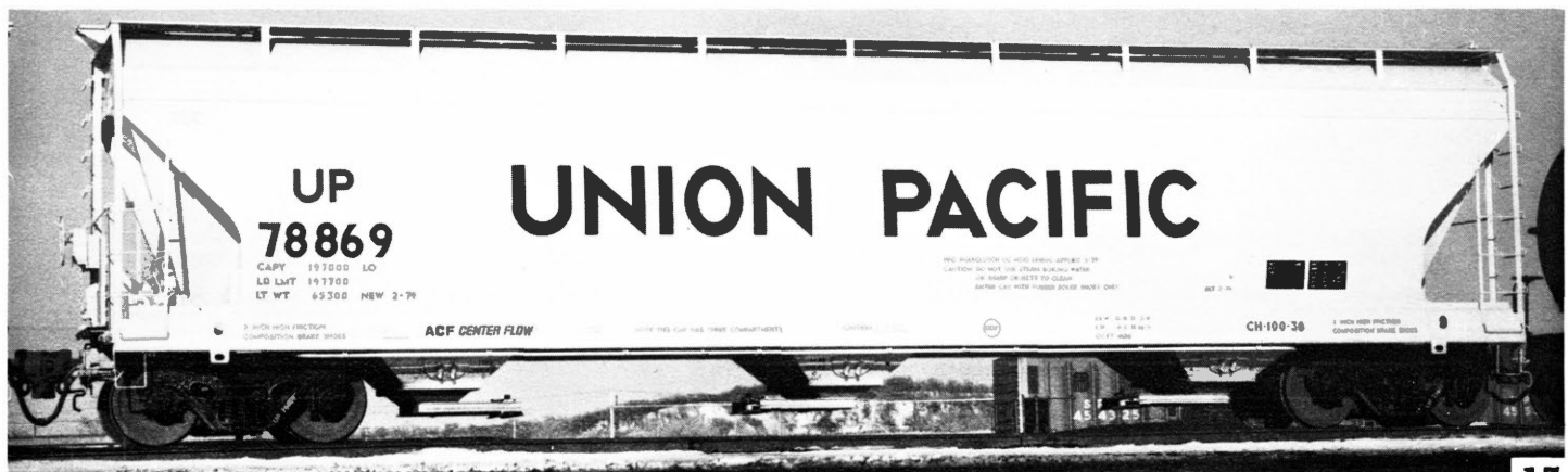
15 78869 class CH-100-38 was built by A.C.F. in 1979 as one of an order for 400 covered hoppers to be used mainly for grain shipments. Photo by G. R. Cockle on 3/5/79 in Council Bluffs, IA.
