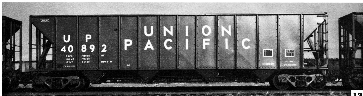
13 40892 class H-100-19 is one of the 850 coal hoppers built by the U.P.R.R. in 1979 at the Albina, OR car shops. Photo by G. R. Cockle in Council Bluffs, IA on 12/17/79.
