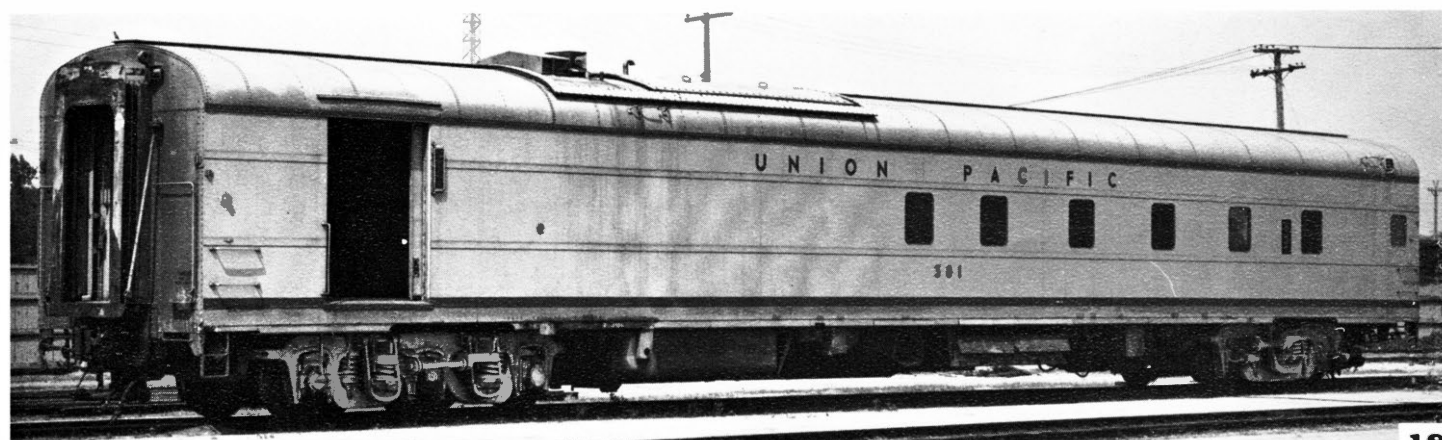
18 301 was originally 6008 built by A.C.F. in 1949 as a Baggage-Dorm. It was converted to a Boiler-Dorm-Baggage in 1962 by U.P.R.R. Photo by G. R. Cockle on 6/5/76 in Council Bluffs, IA.
