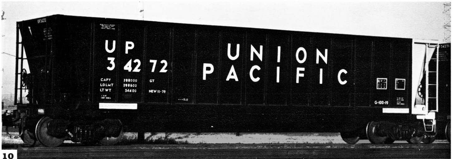
10 34272 class G-100-19 is one of the 600 rotary coal gondolas built by the U.P.R.R. in 1979 and 1980. Photo by G. R. Cockle on 12/19/79 in Council Bluffs, IA.
