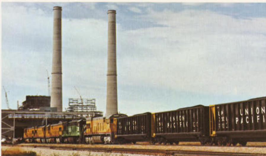
BOTTOM LEFT —Unit coal trains averaging 110 cars each deliver 11,000-ton shipments from Wyoming to the Jeffrey Energy Center near Topeka, Kansas.
